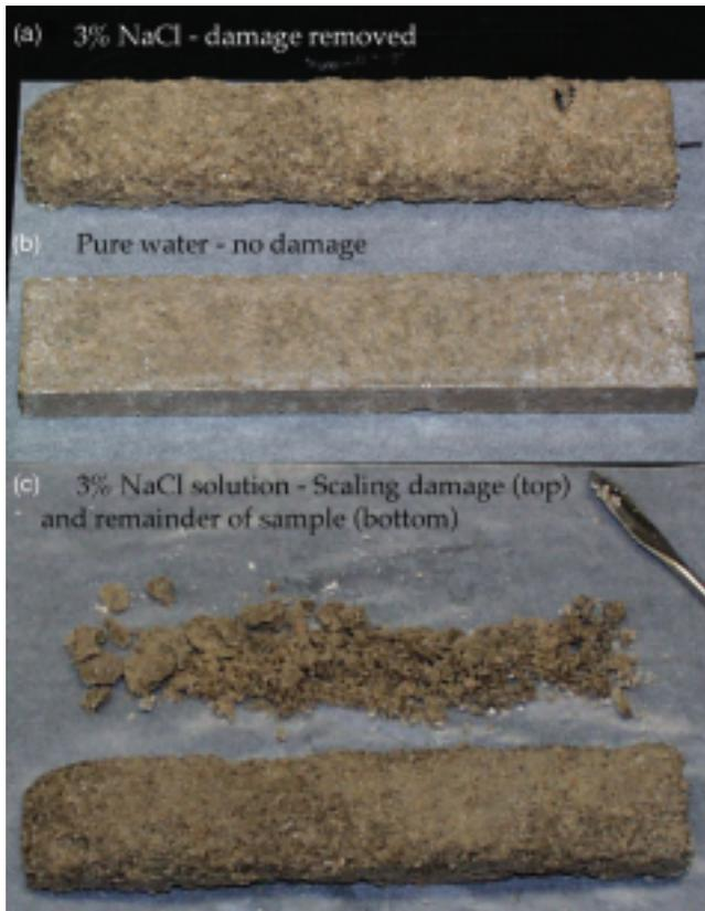
**Fig. 22.** Mortar samples after warping experiments with (a) and (c) 3% NaCl solution, or (b) pure water. (c) Scaling damage removed from the sample is finer than that yielded by the cement paste (Fig. 21). This is a direct result of the interfacial transition zone dominating the fracture process.
