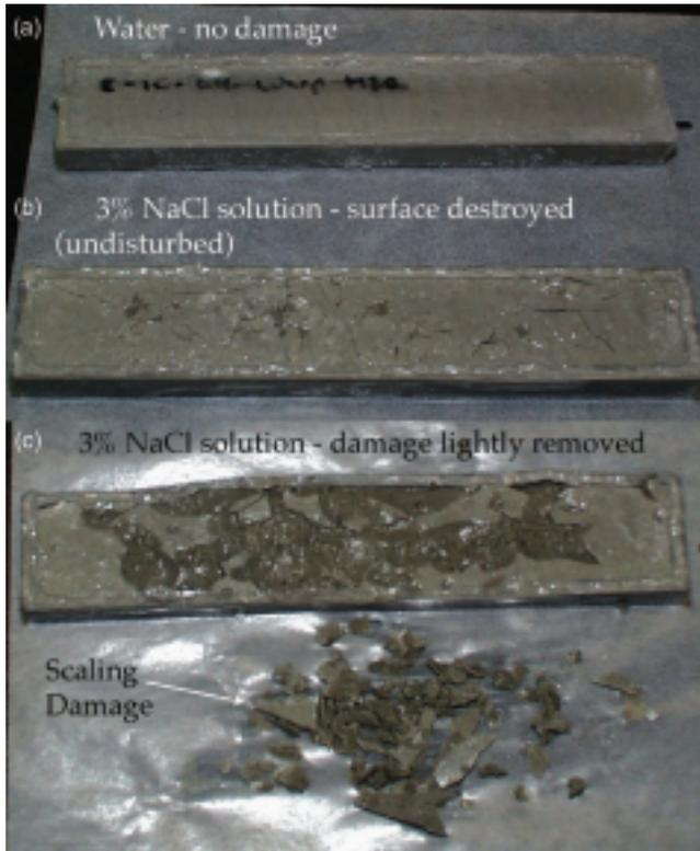
**Fig. 21.** Samples used in comparative warping experiments, the results of which are shown in Fig. 19, clearly illustrate the difference in damage observed with (a) pure water, or (b) and (c) 3% NaCl. The thickness of the scaling damage is ~1–2 mm. The critical stress intensity for a crack propagating parallel to the interface at this depth is  $0.1\text{--}0.25 \text{ MPa} \cdot \text{m}^{-0.5}$ .
