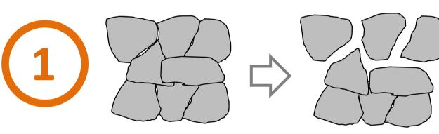
To study the consolidating efficacy of the HAP treatment, artificially aged samples with characteristics similar to naturally sugaring marble (i.e. micro-cracks more diffused near the surface) are needed
