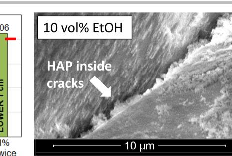
Double application of the HAP treatment with 10 vol% ethanol was able to fully restore the E<sub>d</sub>, thanks to HAP formation inside cracks formed by artificial ageing
