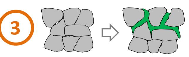
The ability of the HAP treatment to reestablish cohesion between calcite grains and **restore the strength** of weathered marble, without causing overconsolidation, needs to be investigated
