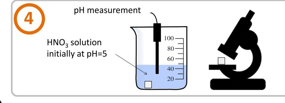
The resistance to dissolution was assessed by measuring the **increase in pH vs time** of an aqueous solution of HNO<sub>3</sub> initially at pH=5 (simulating slightly acid rain)
