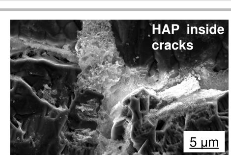
HAP was able to fully restore the modulus of marble preliminarily damaged at 100 °C, thanks to HAP formation inside cracks
