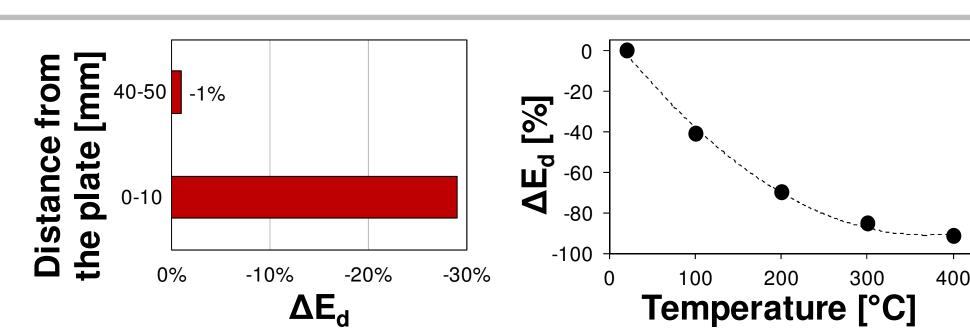
Heating at 200 °C for 20 sec caused near-surface damage similar to that of naturally weathered marble (higher damage at higher temperature)
