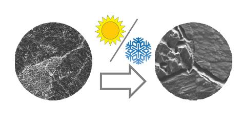
Rain causes the dissolution of calcite grains, so that the marble carved surface is lost
