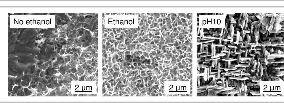
The coverage of marble surface and the new phases morphology were found to be highly influenced by ethanol addition and pH increase
