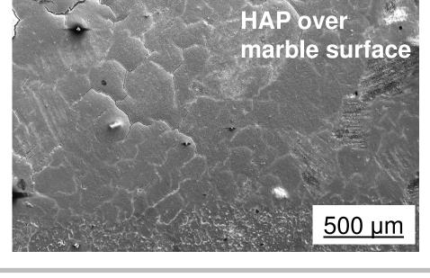
HAP was able to significantly reduce the dissolution of marble (even if the HAP film was cracked at the end of the acid attack test)
