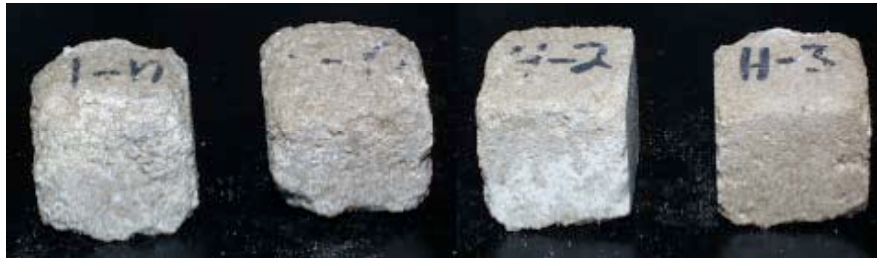
Figure 8. Trial 2 Cycle 16: Untreated stones (left two) and stones treated with PAA-VLMW (right two). Untreated stones begin to round off while the treated stones show only slight deterioration at corners and edges.
