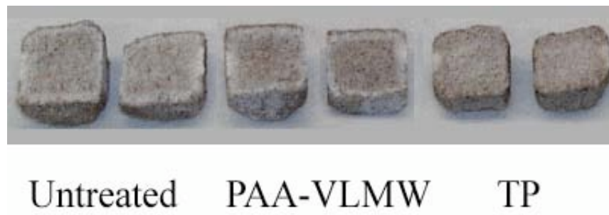
Figure 9. Salt distribution in samples split open after cycle 16 in Series 2. Efflorescence appeared after 10-15 minutes, indicating location of salt. Untreated stone and sample treated with PAA-VLMW has ring of salt within ~1 mm of surface, whereas all salt has retreated to the center of the sample treated with the terpolymer.
